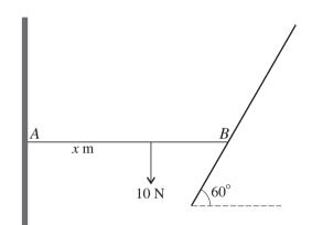
A light rod AB of length 0.8 m has a particle of weight 10 N attached to a point at a distance x m from A. The rod rests in equilibrium in a horizontal position with A against a rough vertical wall and B on a smooth plane inclined at 60° to the horizontal (see diagram). Find, in terms of x, the magnitude of the force that the inclined plane exerts on the rod. [2]
