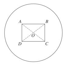
A uniform circular disc has radius 0.5 m, centre O and mass per unit area 6.20 kg m<sup>-2</sup>. A rectangle *ABCD*, where *AC* and *BD* intersect at O, is removed (see diagram). The lengths of *AB* and *BC* are 0.4 m and 0.3 m respectively. Show that the moment of inertia of the resulting lamina, about an axis through *A* perpendicular to its plane, is 0.851 kg m<sup>2</sup>, correct to 3 significant figures. [8]
